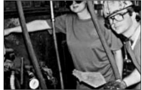
Pyro-Putty® 653 seals Babcock & Wilcox furnace door.
