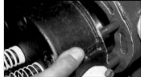
Pyro-Putty® 2400 repairs flanges on a F & J gas engine.
